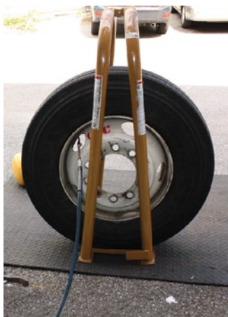
Inflating single-piece rim in restraining device.
